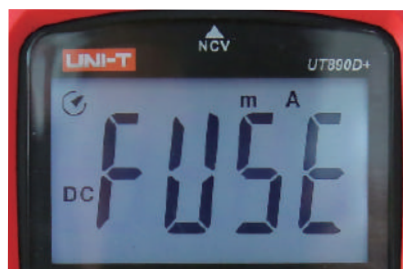
Fuse blowing alarm (mA only)
