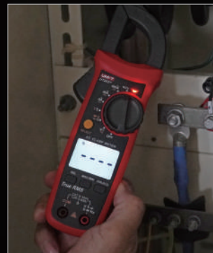
NCV multi-segment display and audio/visual alarm
